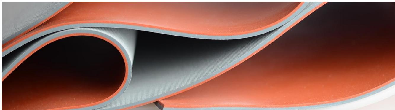
NR 45 Grey/Red - a high-quality, grey-red, multi-layer natural rubber membrane with hardness 45 Shore A. The natural rubber membrane is made in EU from high performed components. The high tear and temperature resistance of material allows to extend service life of membrane. The elastomer NR-45 specially intended for use in membrane presses with positive negative pressure in the woodworking industry. The NR-45 Natural rubber membranes are supplied with cloth/smooth finish.
